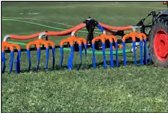
Dribble bar manure applicator displayed at the 2023 FCCD Summer Conservation Farm Tour
